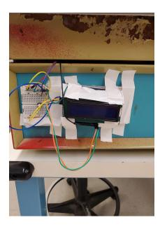
The LCD screen will let the user know the incubator is heating up and will display the current temperature.
